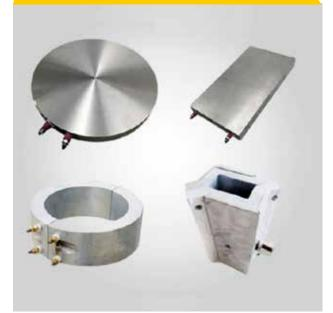
Cast-in heaters are designed for heating solids or indirect heating. Cast-in heating elements are ideal for applications requiring homogeneous indirect heat. Cast-in heaters are often used in plastics industry, packaging industry, food industry and many others. The cast-in heating plates and heating bands consist of one or several electrical resistance embedded in a block of aluminum, brass, bronze or cupronickel alloy.
