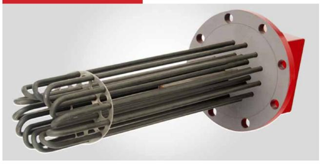
These are the most versatile of all electric heating elements capable of being formed into virtually any configurations. The coil is made up of helically wound coil of Nickel Chrome wire which is housed in a tube of SS 304 Sheath. The space between the coil & tube is filled with specifically selected grain size of high purity Magnesium Oxide (MgO). This increases thermal conductivity, dielectric strength & heater life.
